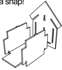
Insert one SIDE PANEL into the BACK vertical slot. Repeat with the other side panel. Insert the SHORT extension of the BOTTOM PANEL into the back horizontal slot.
