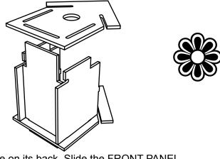
Rest the house on its back. Slide the FRONT PANEL slots over the remaining bottom and side notches. Stand birdhouse upright. Now, press the side panels completly down.
