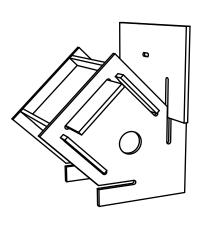
Place the birdhouse on an angle as shown. With the wider ROOF flange toward the front, slide the ROOF panel into place until it locks with the notch.
